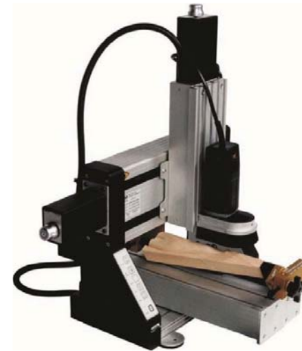
Figure 2-23. DC stepper motors are used on this tabletop educational robot. (Techno, Inc.)
