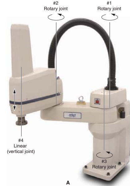
Figure 2-29. A—This is an example of a basic SCARA robot configuration. Note the three rotary joints and the single vertical joint used in this horizontally articulated configuration. B—This is a top view of the work envelope of a typical SCARA horizontally articulated robot configuration. This work envelope is sometimes referred to as the folded book configuration. (Adept Technology, Inc.)
