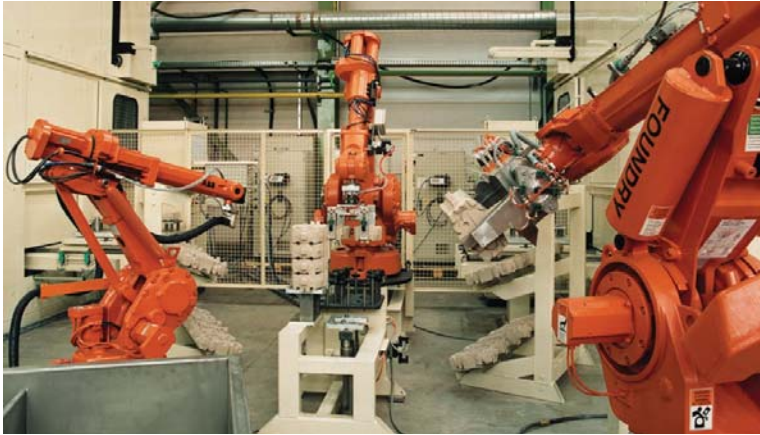
Figure 2-26. Large robots that use hydraulic drive systems perform a demonstration at a manufacturing trade show. (ABB Robotics)
