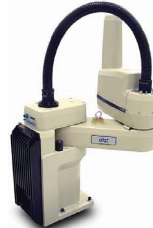
Figure 2-25. Note the simplified mechanical design of this direct-drive robot as compared to the conventional electric-drive robot shown in Figure 2-22 . (Adept Technology, Inc.)
