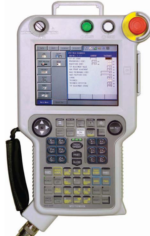
Figure 2-8. This teach pendant is connected to a controller and is used to teach a robot how to complete a task. (Motoman)
