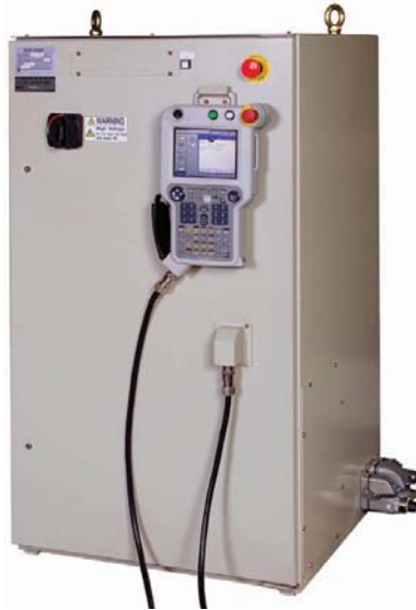
Figure 2-4. A controller/power supply with a teach pendant. (Motoman)
