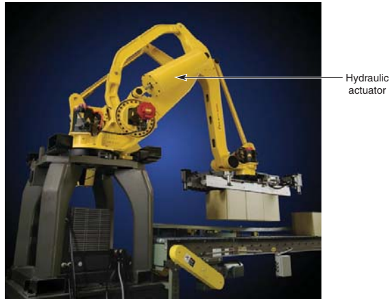
Figure 2-21. A large hydraulic actuator provides up-and-down motion to the manipulator arm of this industrial robot. (FANUC Robotics)
