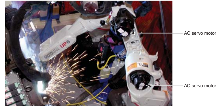
Figure 2-22. This heavy-duty industrial robot uses two ac servo motors in the operation of its manipulator arm. (Motoman)
